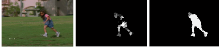
Fig. 2. Positive predictions of each region and the brightness indicates probability of being an object: (a) source image (b) independent SVM predictions (c) predictions from graph transduction capturing the coherent intrinsic structure within visual data, using SVM predictions as input.
